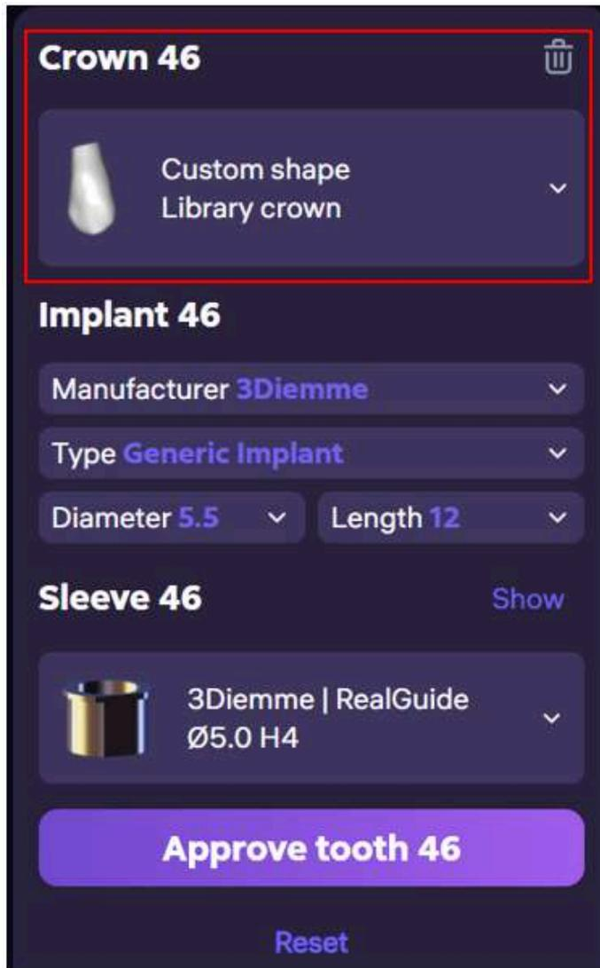
To adjust the shape or position of the digital crown, click on it on the 3D scene. Object controls will appear, the orientation of the controls is dependent on the camera angle.
